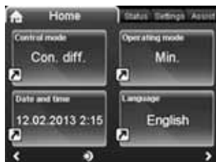
Fig. 16 Example of main display on a TPE Series 2000 with advanced control panel
