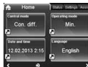
Fig. 1 Example of main display on a TPE Series 2000 with advanced control panel
